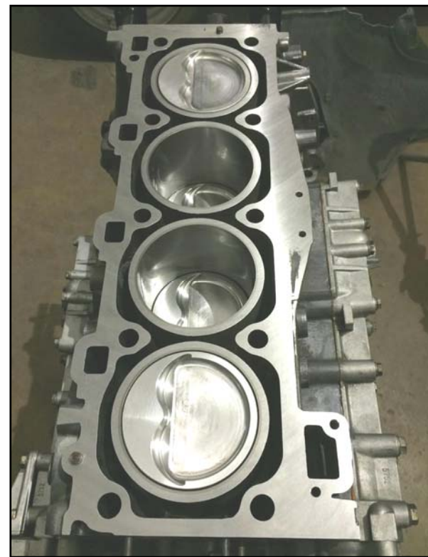
Dry sleeved and bored to just over 102 millimeters. JE small block Chevy pistons, forged 4032. Eagle 150 millimeter Mitsubishi rods. 86 millimeter stroke cross drilled crank, 8.1:1 compression.
