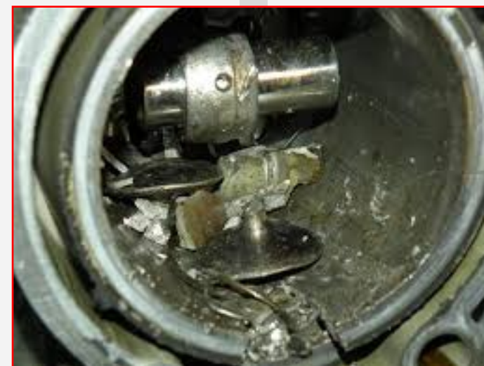
"An IMS failure spews metal throughout the engine."
