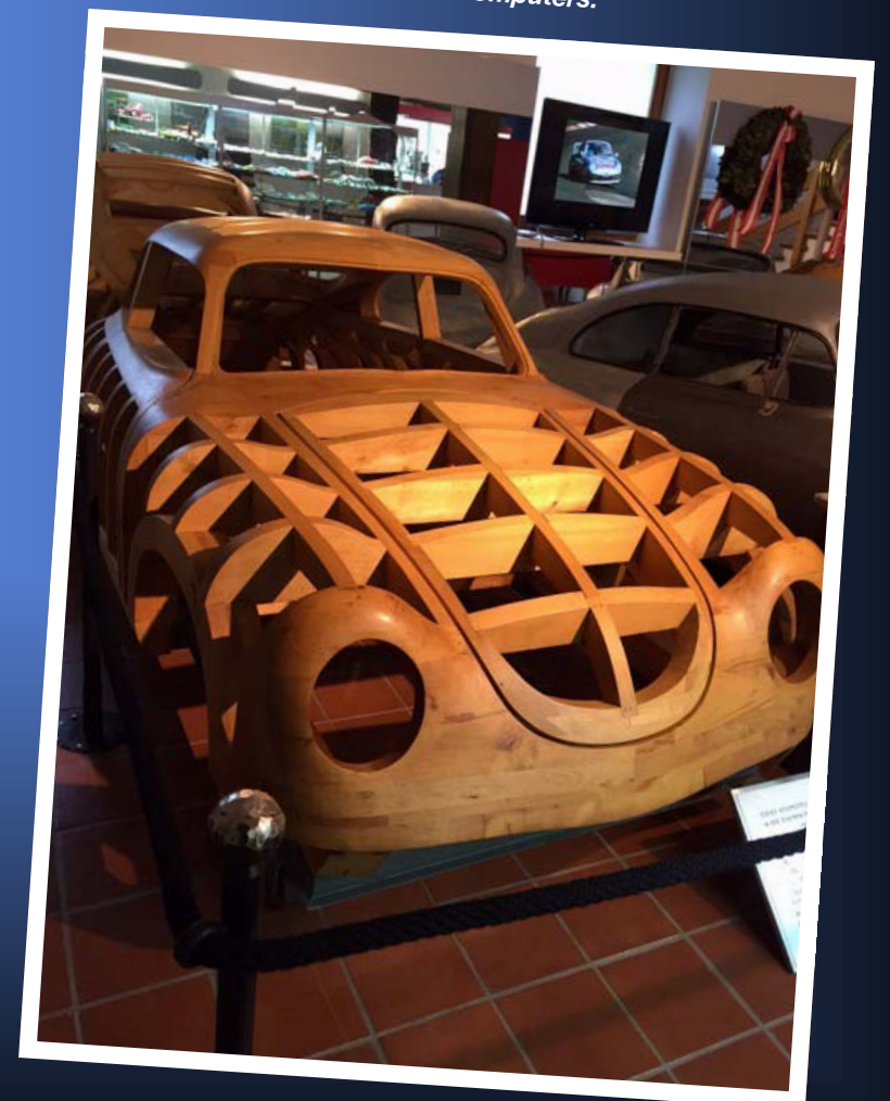
356 body buck at Gmund - the way cars were designed before computers.
